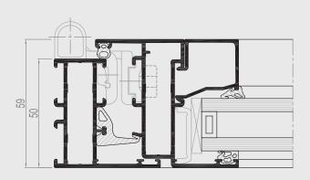
CS 59Pa offers an extensive range of non-insulated profiles for the construction of elegant and moderately priced aluminium frames in functional style. Therefore CS 59Pa is the ideal system for outdoor applications in warm climates but it can also be used for the partitioning of indoor office spaces.
