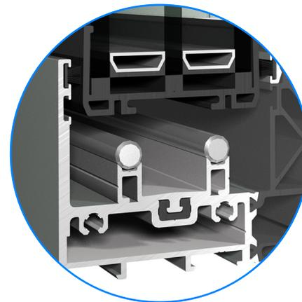
Designed for triple-glass configurations with standard depth\*, it reduces operating forces by **30-50%** while providing a **maintenance-free, durable, and futureproof solution**. The new hardware is easy to retrofit, simply replacing the rail and wheels, making it ideal for existing HiFinity triple glass configurations.
